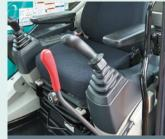
Double slides allow adjustment for optimum comfort
