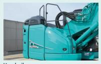
Handrail The handrail on the step side allows easy access to the maintenance port on the upper arm.
