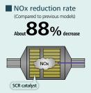
At high temperatures, nitrogen and oxygen combine to produce nitrous oxides (NOx). Reducing the amount of oxygen and lowering the combustion temperature results in much less NOx.
