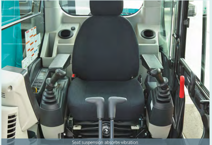
Seat suspension absorbs vibration
