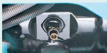
Engine oil quick-drain valve can be turned without special tool.
