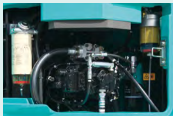
Fuel filter with built-in water-separator
