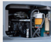
● Firewall separates the pump compartment from the engine
