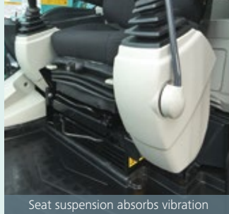
Seat suspension absorbs vibration
