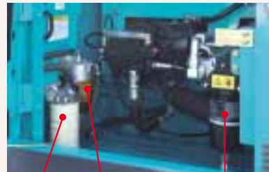
Main fuel filter Pre-fuel filter (with built-in water separator) Engine Oil Filter
