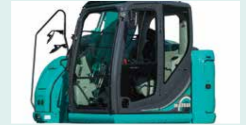
Mounting brackets for vandalism guards are standard equipment (contact your KOBELCO dealer to fit vandalism).
