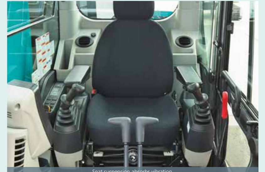
Seat suspension absorbs vibration
