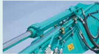
Dismantling bucket cylinder
