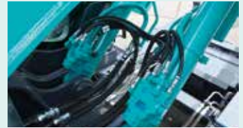
Boom & arm holding valves
