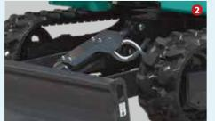
Blade Cutting Edge Backfill dozer blade has wear-resistant cutting edge.
