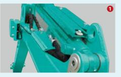
Dozer Dozer cylinder rod guard protects dozer cylinder from damage.
