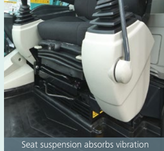
Seat suspension absorbs vibration
