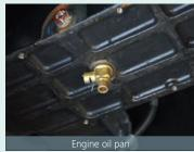
Engine oil pan equipped with drain valve.
