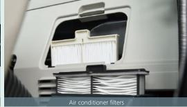
Internal and external air conditioner filters can be easily removed without tools for cleaning.
