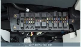
More finely differentiated fuses make it easier to locate malfunctions.
