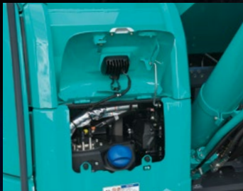
Ground level DEF tank
