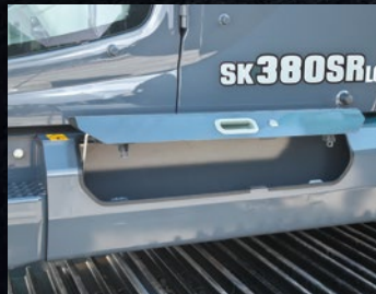
Ground level storage compartment access
