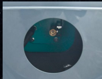
Remote fuel tank drain valve
